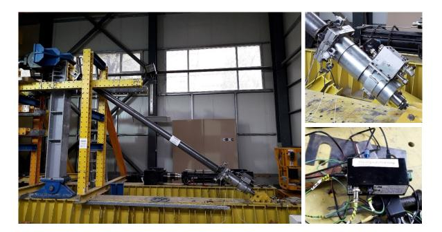
The experimental tests have demonstrated the functionality of this system, but in order to optimize the way it works – there are several aspects of detail to be solved. The functionality of the hybrid system has been demonstrated in the sense that it has highlighted how the dampers work in a first phase, then by electronical control at the work capacity, the damper was blocked and the buckling restrained brace was operating.
